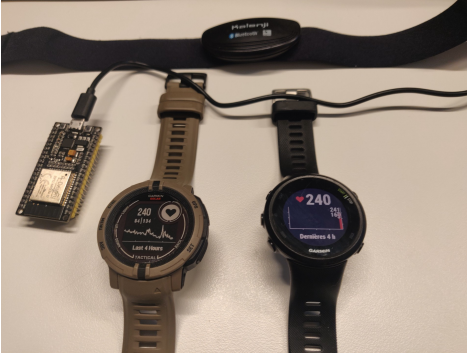
Fig. 7. Experimental setup for malicious ANT+ packet injection.
