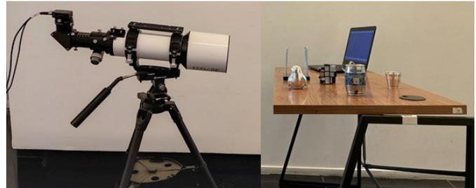
Fig. 1: A photodiode is mounted on a telescope (left) and directed at a shiny object on a desk (right). The photodiode is used to obtain optical measurements from the light reflected from the shiny object’s minuscule vibrations induced by sound.
